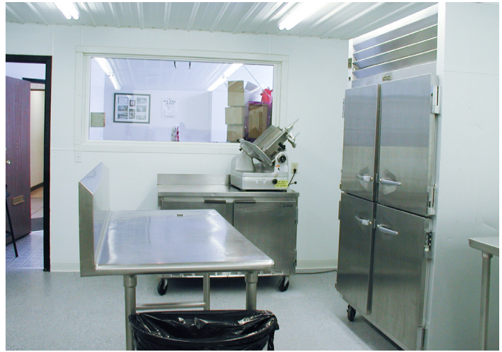
This room in a processing facility has adequate lighting and acceptable floor, wall, and ceiling materials.
