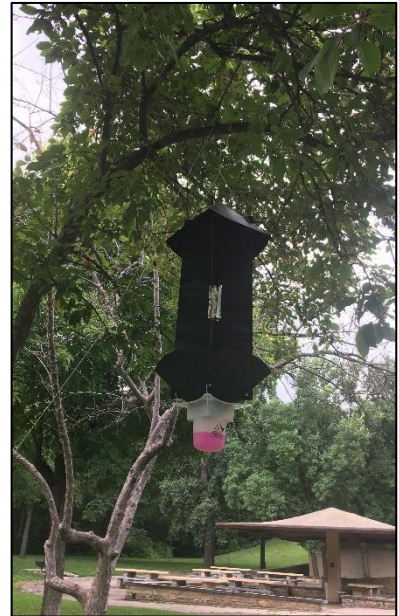
Figure 11. A cross-vane trap is used for VLB detection surveys.
