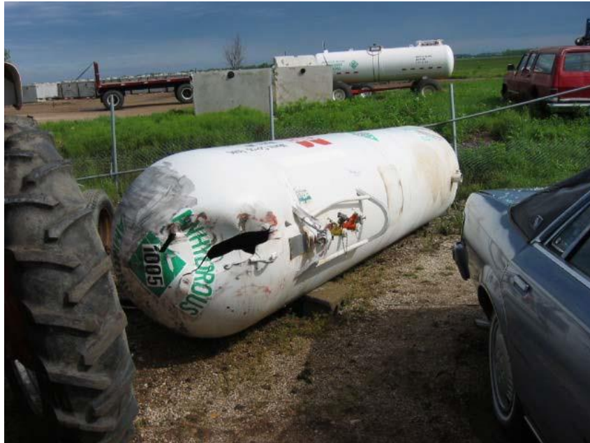
Front of nurse tank showing black rubber tire marks and red paint from when the tank struck the tractor. Dent and opening also caused by collision.
