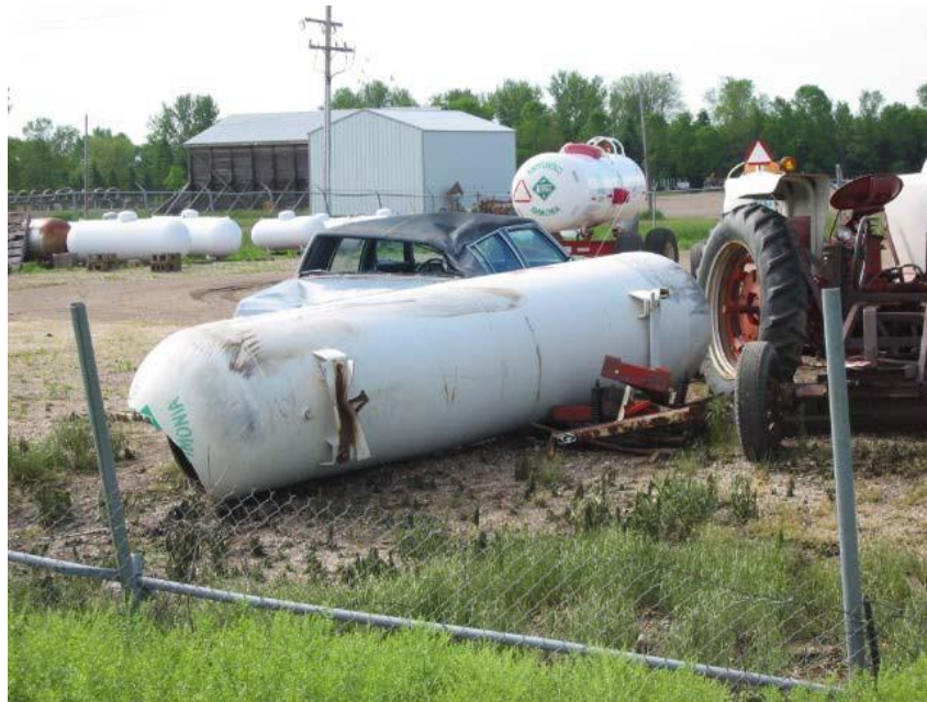
Running gear absent. Gear remained at load-out risers.
