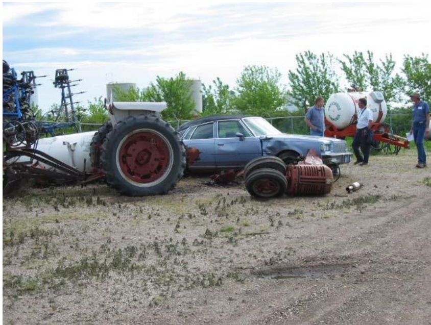
Tank split apart this tractor before finally coming to rest on its side.
