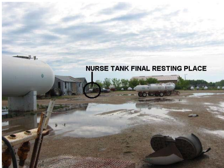
Final resting place of the nurse tank approximately 250 feet away. Part of the tank shell is located in the lower right portion of the photograph.
