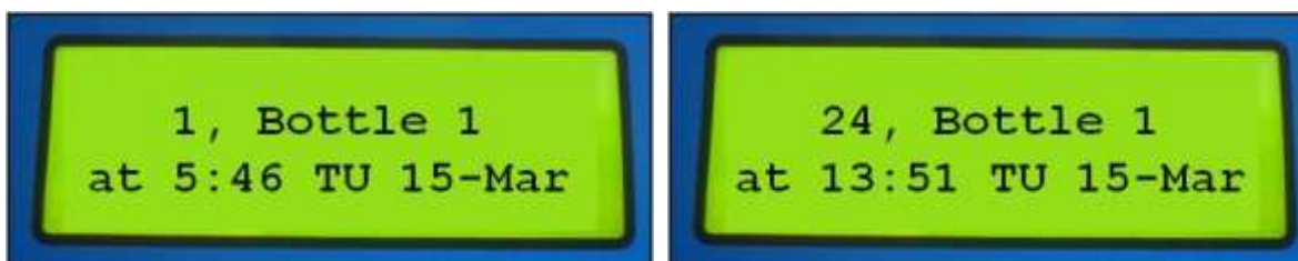
Figure 9. Pulse #, Bottle #, and sample date and time readout of the ISCO 6712 Automatic Sampler. The two images above represent the start and stop times for bottle #1.
