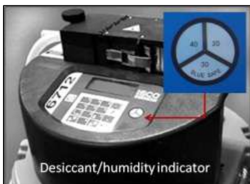
Figure 18. Location of humidity indicator card on the ISCO 6712 autosampler.
