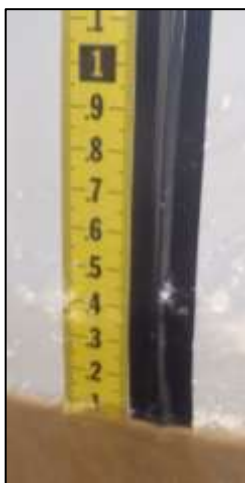
Figure 1. Flume staff gage.
