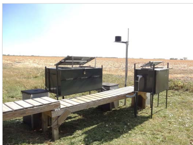
Figure 2. Subsurface Drainage Monitoring Station
