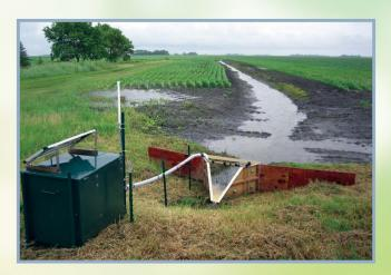
In addition, precipitation and air temperature are continuously measured. Soil moisture and soil temperature are measured near the surface drainage monitoring station.
