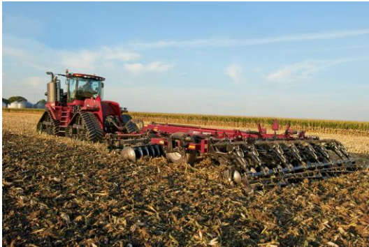
Figure 17. Typical conservation tillage ripper with discs.
