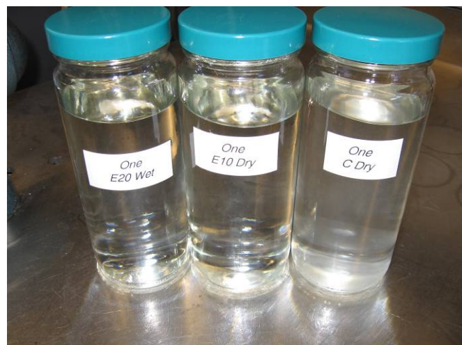
Figure 9. Cloudiness caused by ACM in Fuel C
