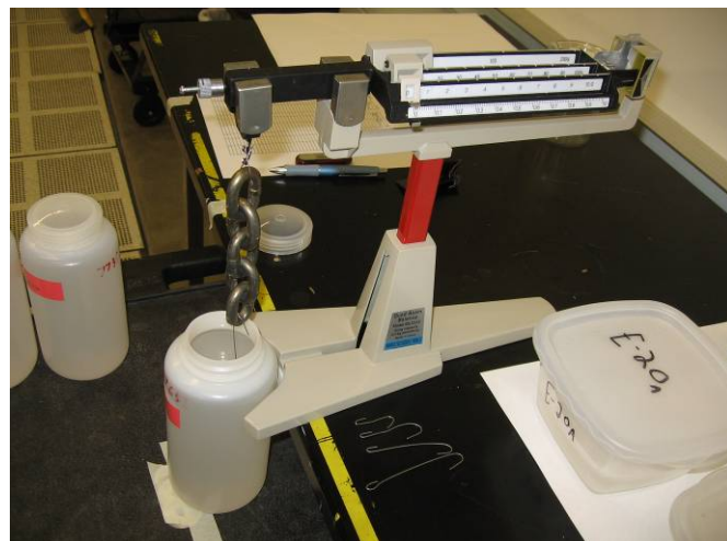
Figure 3. Quad beam balance used for volume measurements
