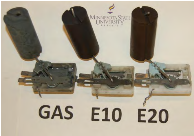
Figure 7. Comparison of residue coatings and discoloration after 4000 hours
