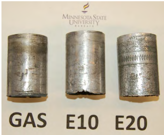
Figure 4. Comparison of pump housings after 4000 hours; note the light surface corrosion on the E20 housing
