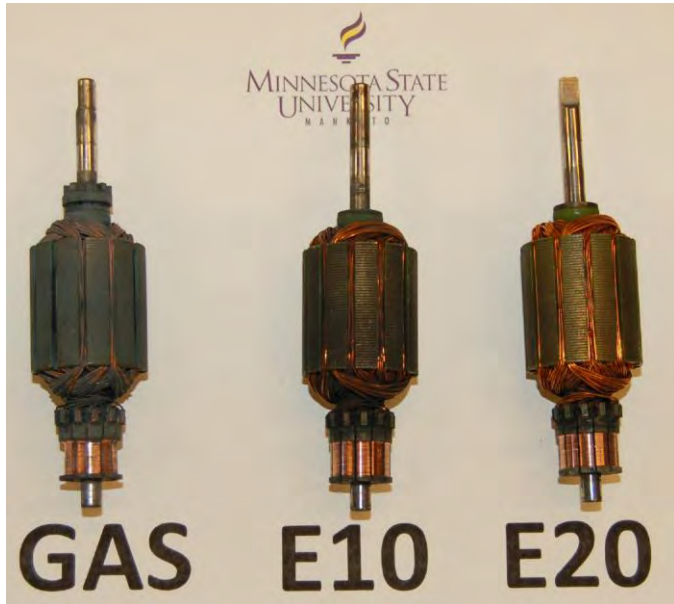
Figure 3. Comparison of residue on armatures after 4000 hours; note commutator wear on the one tested in gasoline
