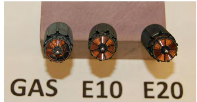
Figure 6. Comparison of armature wear after 4000 hours; note the commutator is worn through to the insulation on the one tested in gasoline
