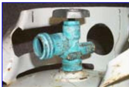
Twenty-pound propane tank galvanized valves will corrode, turn blue and weaken from exposure to AA vapor and/or liquid. Never move a suspected
