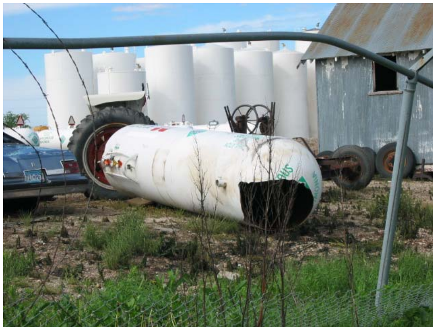
Large opening where the tank failed. Absent shell piece remained by load out risers.
