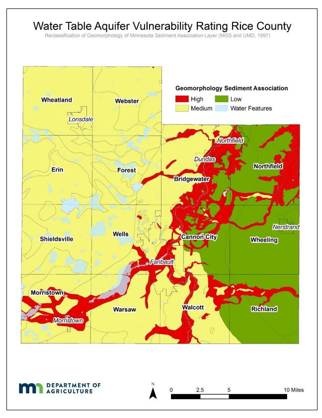
Figure 4. Water Table Aquifer Vulnerability Rating in Rice County
