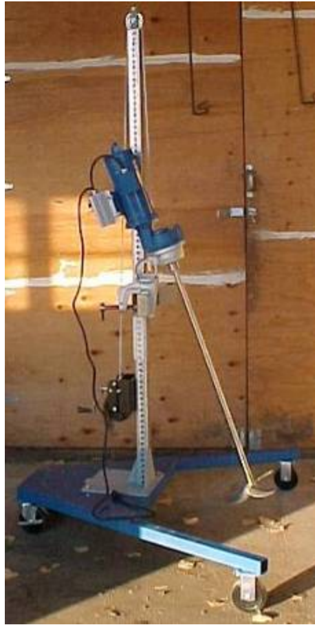
Figure 59: A Grovhac \frac{3}{4} horsepower, variable speed prop mixer, and a plastic barrel were the primary tools for mixing liquid manure.
