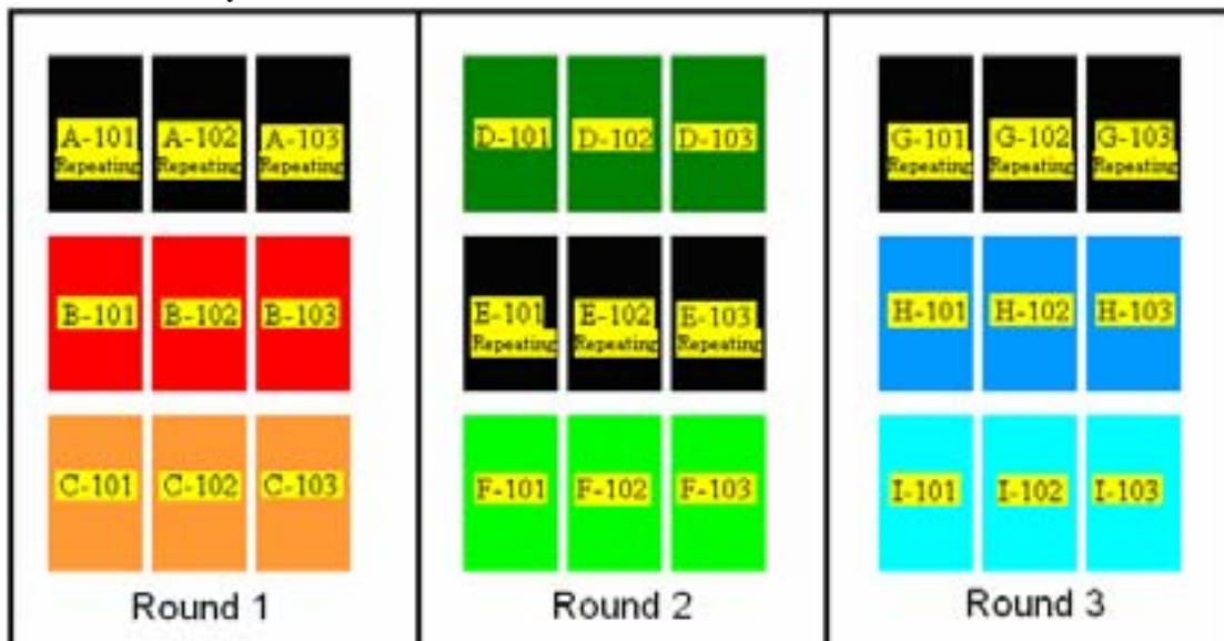
Figure 34: Three rounds of samples. Samples A, E, and G are the same sample so results can be compared from round to round. Triple replicates (101, 102 and 103) allow evaluation for precision in addition to accuracy.
