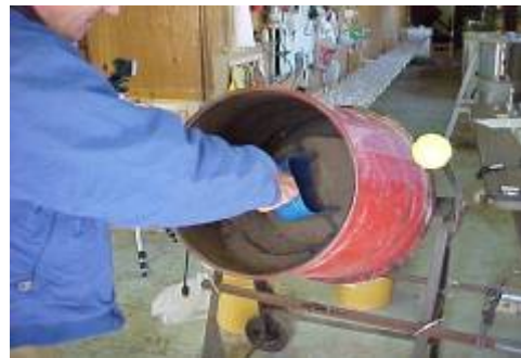
Figures 16 and 17: A smaller mixer was used for some solid samples before the Imer mixer was purchased. This mixer was non-project equipment.
