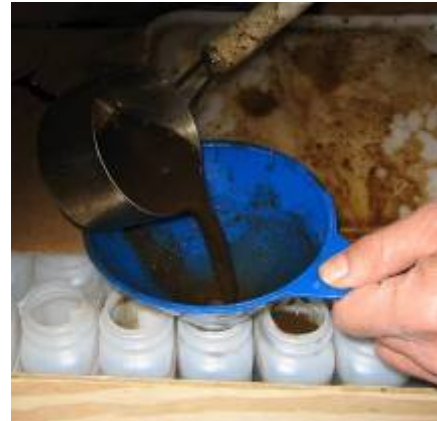
Figures 65 and 66: A ladle and funnel proved to be the most efficient method for filling sample bottles with liquid manure. Cardboard and a plastic lid reduced manure drips on the bottles.
