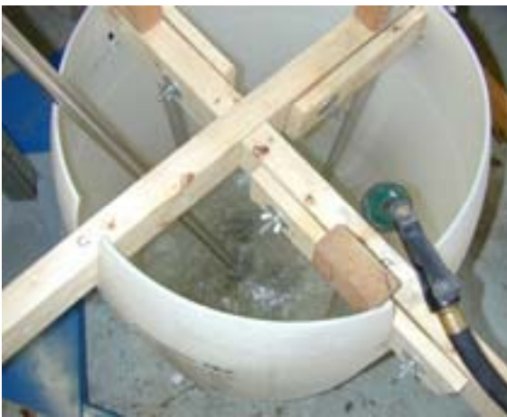
Figures 60 and 61: Water and baffles are added to the mixing barrel (50 gallon barrel in picture). Solid manure that had been processed with water in the Robot Coupe VCM is added to the mixing barrel while the prop mixer is running.
