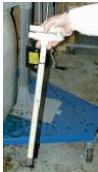
Figures 69 and 70: A dip tube was tried one time and quickly abandoned. It was messy, slow, and the sample homogeneity was not as good as other methods.
