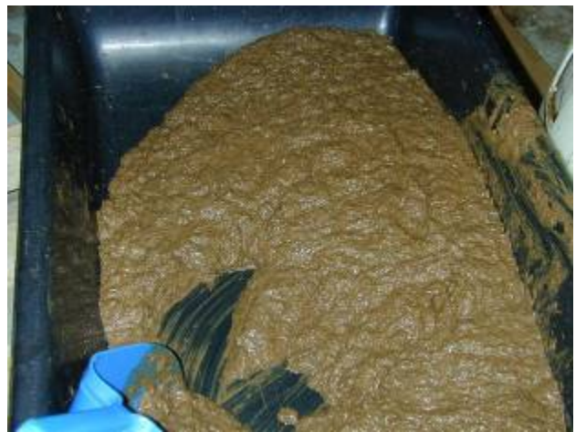
Figures 60 and 61: Water and baffles are added to the mixing barrel (50 gallon barrel in picture). Solid manure that had been processed with water in the Robot Coupe VCM is added to the mixing barrel while the prop mixer is running.
