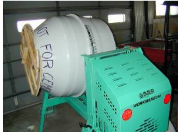
Figures 14 and 15: Solid manure is mixed in the Imer Workman 350E Electric cement mixer, a 12 cubic foot mixer. A wooden cover keeps the dust contained within the mixer.
