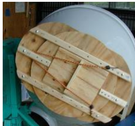
Figures 48 and 49: A wooden cover on the cement mixer reduces dust.
