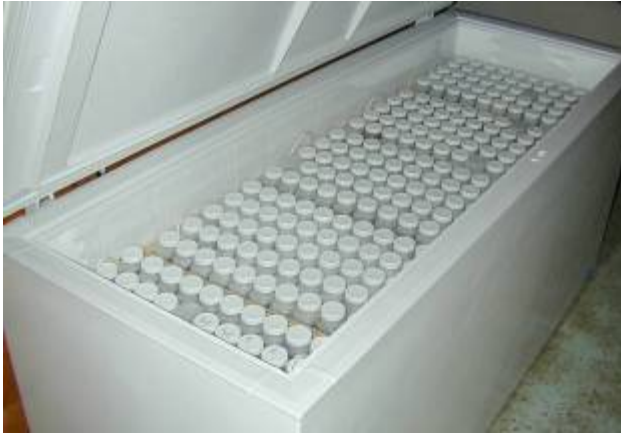
Figures 27 and 28: Trays that fit snugly maximize the freezer capacity. Three smaller trays (30 bottles) fit over the freezer motor and compressor. Five larger trays (50 bottles) fit from top to bottom. A full freezer holds 1,090 sample bottles – more than enough for one exchange.
