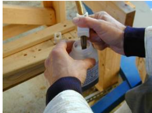
Figures 67 and 68: A siphon tube was the fastest and cleanest method for filling the sample bottles with liquid manure. However, solids can cause the tube to clog and the clogs may act as a filter and reduce the sample homogeneity. This method was attempted several times and finally abandoned in favor of using a ladle.
