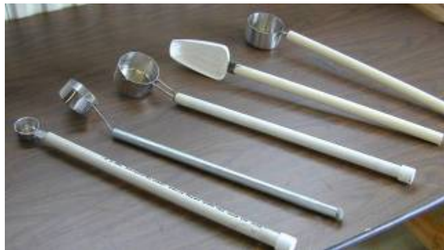
Figure 64: Various sized and shaped ladles were used to fill the sample bottles for both liquid and solid manure.
