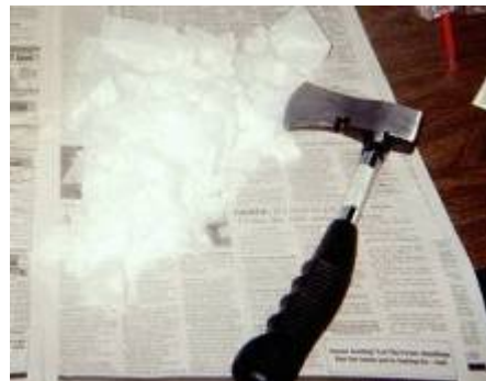
Figures 38 and 39: The finest particle size was obtained by processing frozen manure with dry ice. A six to eight pound block of dry ice is split in half and then chopped into finer pieces.
