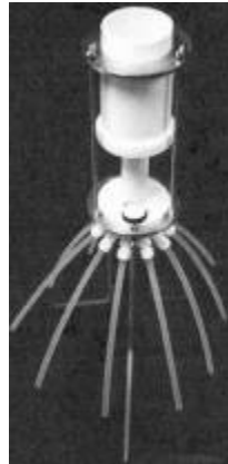
Figure 33: Dekaport cone Teflon sample splitter (the hoses were too small and quickly clogged with manure solids)
