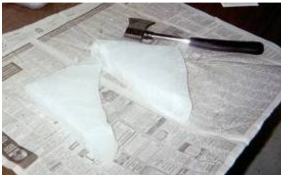
Figures 38 and 39: The finest particle size was obtained by processing frozen manure with dry ice. A six to eight pound block of dry ice is split in half and then chopped into finer pieces.
