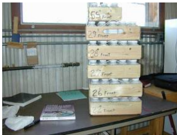
Figures 82 and 83: Each sample set consists of five large trays (50 bottles/tray) and one small tray (30 bottles) for a total of 280 bottles. Each lab received three replicates for analysis and 20 bottles were analyzed to check homogeneity. That left about 50 bottles of each manure sample for the manure sample repository.
