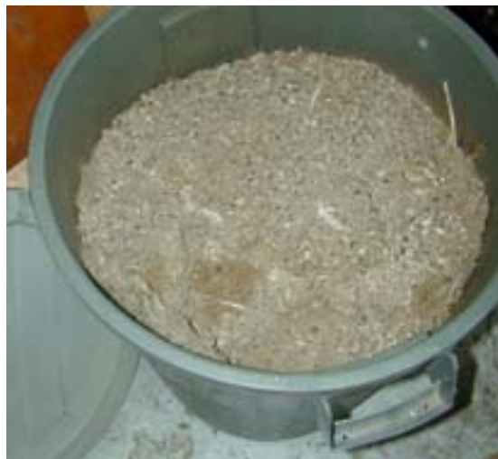
Figure 36: Thirty-two gallon garbage can of solid manure (turkey litter) before processing. This is enough for a single sample set (280 bottles).
