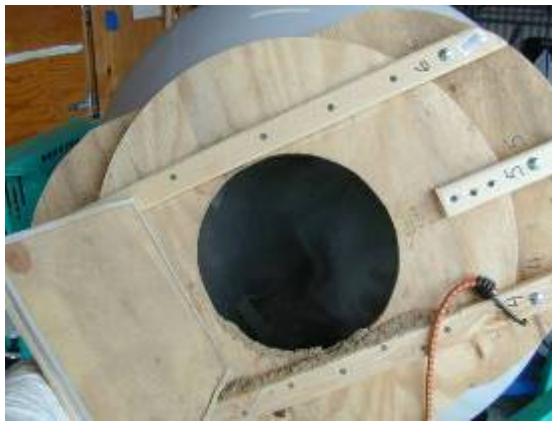
Figures 48 and 49: A wooden cover on the cement mixer reduces dust.
