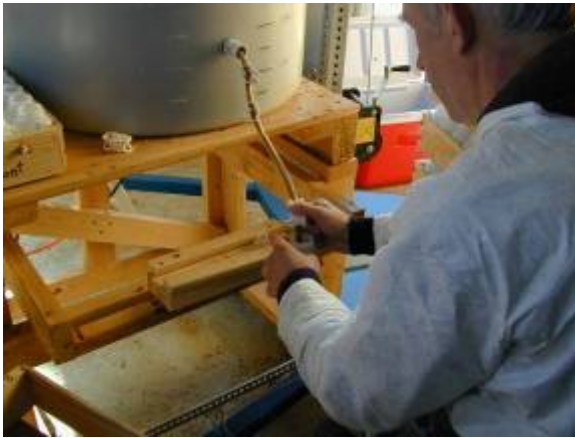
Figures 67 and 68: A siphon tube was the fastest and cleanest method for filling the sample bottles with liquid manure. However, solids can cause the tube to clog and the clogs may act as a filter and reduce the sample homogeneity. This method was attempted several times and finally abandoned in favor of using a ladle.
