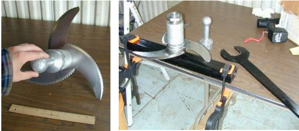
Figures 5 and 6: Serrated knife blades produced better results than smooth blades. The large wrench and the arbor holder were fabricated by a local blacksmith.
