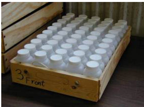
Figures 82 and 83: Each sample set consists of five large trays (50 bottles/tray) and one small tray (30 bottles) for a total of 280 bottles. Each lab received three replicates for analysis and 20 bottles were analyzed to check homogeneity. That left about 50 bottles of each manure sample for the manure sample repository.
