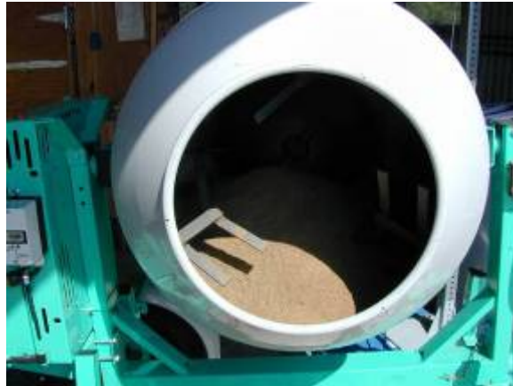
Figure 47 Step 3 — After processing in the Robot Coupe VCM, the manure is mixed in the large Imer cement mixer.
