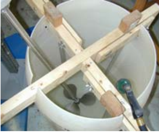
Figures 12 and 13: The 50 gallon mixing tank is on the left and the 100 gallon mixing tank is on the right. Aluminum baffles were added to aid mixing.
