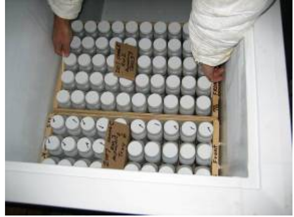
Figures 27 and 28: Trays that fit snugly maximize the freezer capacity. Three smaller trays (30 bottles) fit over the freezer motor and compressor. Five larger trays (50 bottles) fit from top to bottom. A full freezer holds 1,090 sample bottles – more than enough for one exchange.
