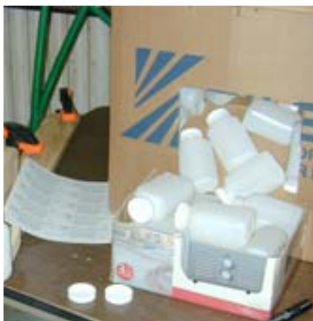
Figure 81: A simple hopper made from a couple of cardboard boxes used along with the labeling jig speeds up the labeling process.
