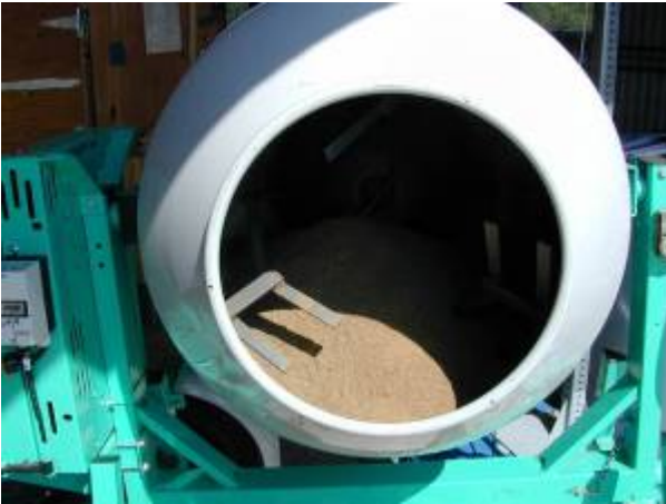
Figures 14 and 15: Solid manure is mixed in the Imer Workman 350E Electric cement mixer, a 12 cubic foot mixer. A wooden cover keeps the dust contained within the mixer.
