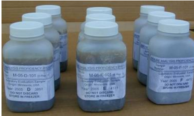
Figure 35: One set of Samples D, E, and F ready to ship to a participating laboratory for the second round of 2005. Each sample has three replicates labeled 101, 102, and 103. The bottles are 250 ml and contain about 200 ml of manure.
