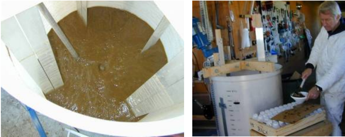
Figures 62 and 63: Additional water and manure processed the Robot Coupe VCM are added to the mixing barrel while the mixer runs. The 100 gallon mixing barrel is shown in these pictures.
