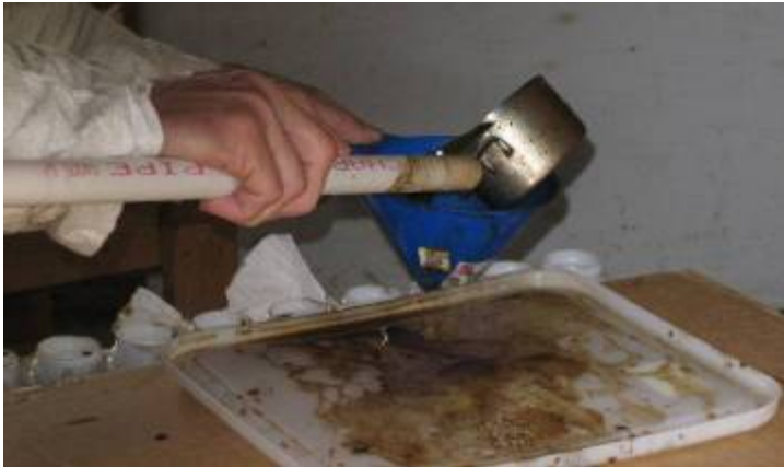
Figures 65 and 66: A ladle and funnel proved to be the most efficient method for filling sample bottles with liquid manure. Cardboard and a plastic lid reduced manure drips on the bottles.
