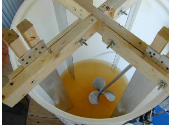
Figures 12 and 13: The 50 gallon mixing tank is on the left and the 100 gallon mixing tank is on the right. Aluminum baffles were added to aid mixing.
