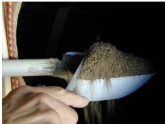
Figures 50 and 51: The fastest and most homogeneous samples (based on MDA lab homogeneity results) were produced by taking the sample directly from the cement mixer and using a large enough ladle to fill the sample bottle in one pass.
