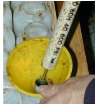
Figures 69 and 70: A dip tube was tried one time and quickly abandoned. It was messy, slow, and the sample homogeneity was not as good as other methods.
