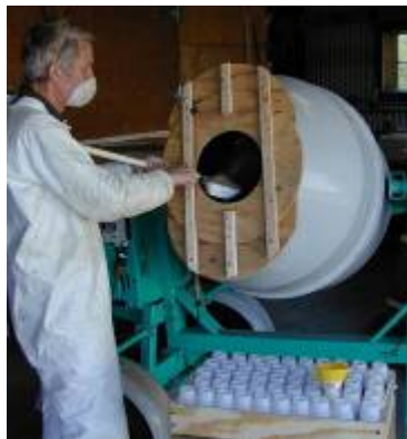
Figures 50 and 51: The fastest and most homogeneous samples (based on MDA lab homogeneity results) were produced by taking the sample directly from the cement mixer and using a large enough ladle to fill the sample bottle in one pass.
