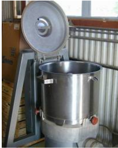
Figure 37: Step 1 — Process manure in the Robot Coupe VCM to reduce particle size.
