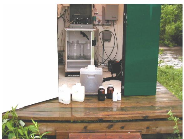
Figure 1. Monitoring station on the Le Sueur River showing refrigerated autosampler for the collection of composite samples.
